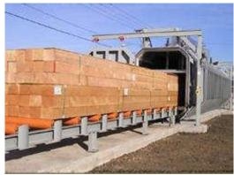
Radio Frequency (RF) is a range of electromagnetic waves between audio and infrared, much like a cell phone. An amplifier is used to generate RF at a fixed frequency which allows control of the heat keeping the kiln at a consistent temperature throughout the process. Prior to being exposed to the RF waves, water molecules are not aligned. When RF is introduced to the wood, the water molecules will excite, align, and exit the wood through the natural veins water traveled while the tree was alive.
